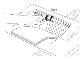
3 Insert the tab on the end of the media guide arm into the slot.
